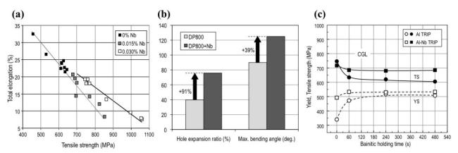
Fig. 6. (a) Effect of Nb addition on property balance in low-carbon DP800 steel (0.08%C-2.0%Mn-0.5%Cr); (b) Effect of Nb induced grain refinement on hole expansion and bending behavior in DP800 steel; (c) Property balance in TRIP steel (0.2%C-1.5%Mn-2.0%Al-0.045%Nb) in function of bainitic holding.
