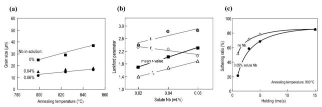
**Fig. 5.** Effects of adding Nb to a Ti-stabilizes IF high strength steel (0.003%C-0.002%N-0.07%Ti-Mn-P); (a) Evolution of final grain size in function of annealing temperature at various solute Nb levels; (b) Evolution of r-value in function of the solute Nb level; (c) Softening behavior for annealing close to the  $A_{r1}$  temperature.
