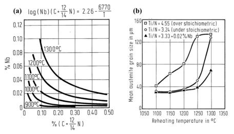
Fig. 2. (a) Solubility isotherms of Nb as a function of C and N in austenite; (b) Effect of non-dissolved particles on the austenite grain size during slab reheating.
