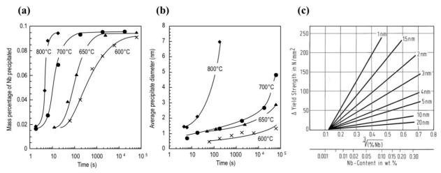
Fig. 4. Precipitation behavior of hot rolled strip with 0.03%C-1.7%Mn-0.1%Nb after low temperature coiling; (a) Fraction of precipitated solute Nb after annealing treatment at various temperatures and times; (b) Coarsening behavior of NbC precipitate depending on annealing temperature and duration; (c) Influence of NbC precipitate amount and average size on yield strength increase.
