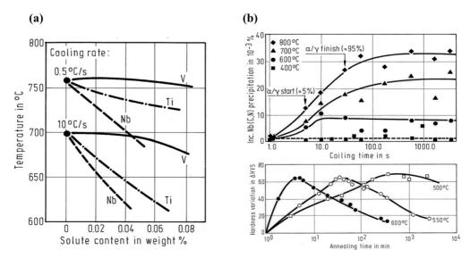
Fig. 3. (a) Dependency of  $A_{r3}$  temperatures on solute microalloying content in 0.1%C-1.5%Mn steel with standard austenite grain size of 100  $\mu$ m; (b) Effect of isothermal holding on Nb precipitation in 0.04%C-0.5%Mn-0.04%Nb steel.
