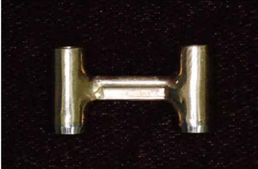
Fig. 2. Reference framework casted with gold alloy
