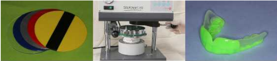
Fig. 1. (a) Ethylene vinyl acetate sheet, (b) duromate-TE, Signature Mouthguards System (Dreve Dentmid gmbH, Unna, Germany) (c) Laminate type mouthguard
