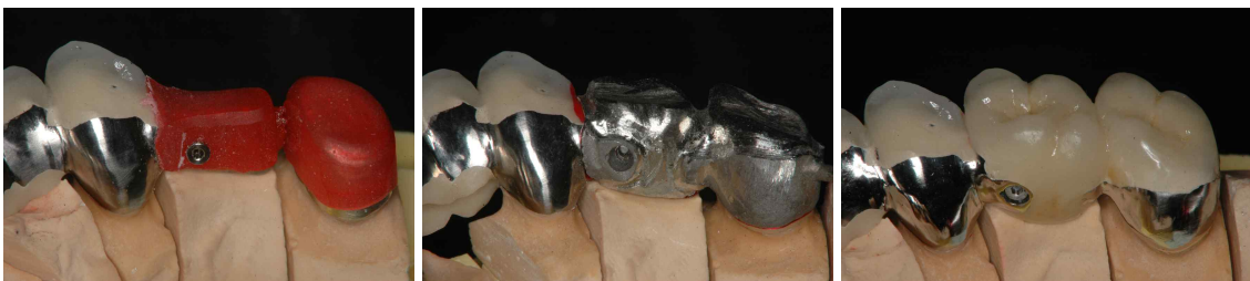
Fig. 10. #25 and #26 outer crowns are connected to the #23 distal bar with Lingual set screw
