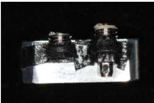
Fig. 2. Fixed specimens with conductive carbon fiber.
