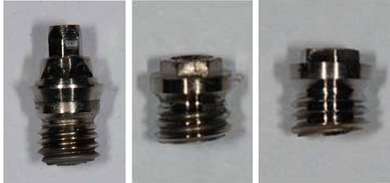
Fig. 1. Upper part of fractured implant fixtures.
