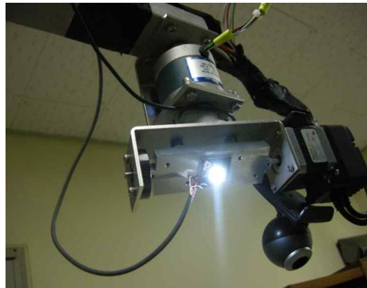
Fig. 6. Tilting Head Light System : In the 2-Axis Tilting Head, a Stepping Motor (Ez-Step 42, Autonics, Korea) was used.
