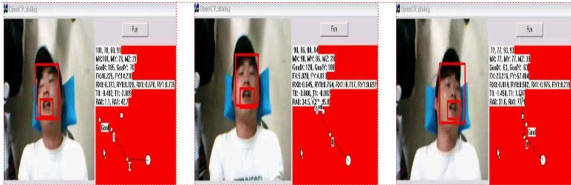
Fig. 10. Result pictures of the face detection : Following the experiment on the detection of facial images, the location of oral cavity could be detected.
