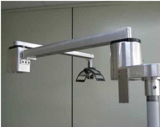
Fig. 5. 2-Linked Arm : 2-Linked Arm requiring a higher degree of the torque, a 5-phase Stepping Motor (AK-M566W-RB5, Autonics, Korea) with a decreased rate ratio of 10:1 was used.
