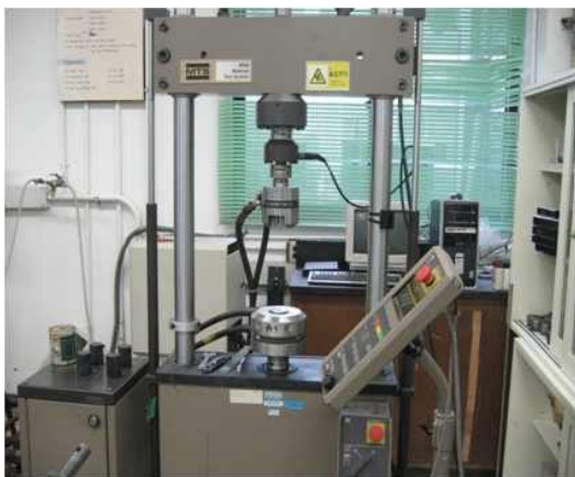
Fig. 5. Loading machine (MTS 810, Material Test Systems Co., Minnesota, U.S.A.)
