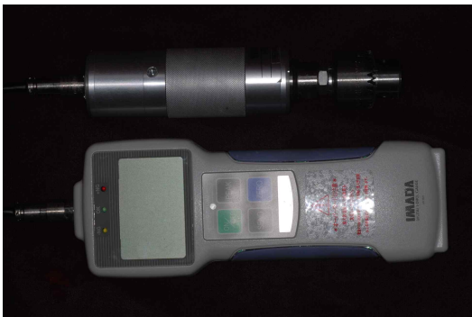
Fig. 4. Digital torque gauge (HTG2-200Nc, IMADA Co., JAPAN)
