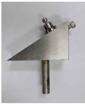
Fig. 1. Customized jig for cyclic fatigue loading test
