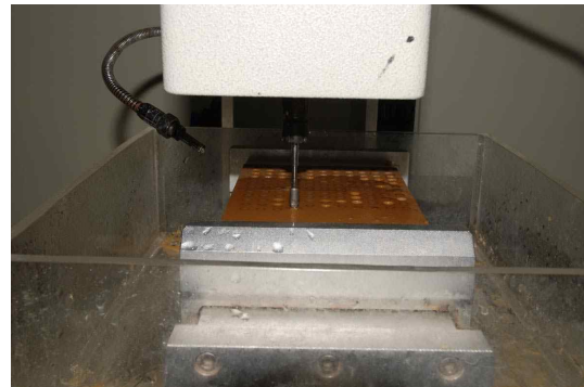
Fig. 4. Forming of insertion hole with auto drilling machine.
