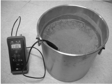
Photo 1 pH of recycled aggregates elution and equipment
