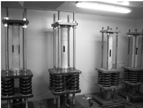
Photo 1 Apparatus for Creep Test
