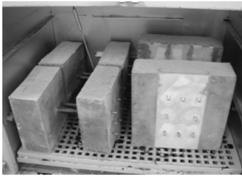
Photo 3 Test set-up of bond properties according to thermal conditions
