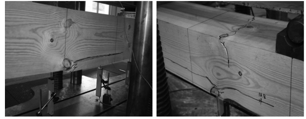
Fig. 9 Failure phenomenon of flexural Specimens
