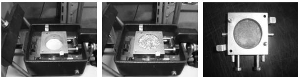
Fig. 7 Direct shear test of concrete and crushed stone
