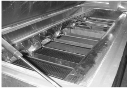
Fig. 1 Water-freezing and water-thawing test
