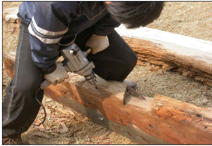
Fig. 3. Coring the samples replaced during repairing process.
