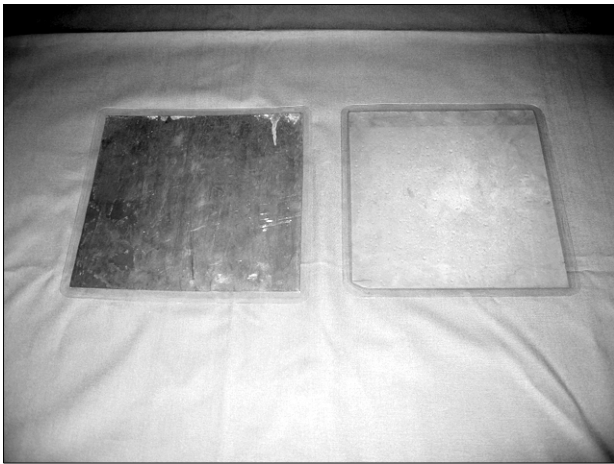
Fig. 3. The Pb 0.5 mm thickness of filter for standard (Left) and experimental lead-free shielder (Right) which is 200×200×1.5 mm 3 of size for 0.42 mm Pb equivalent.
