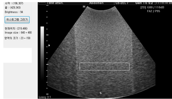
Fig. 1 Measurement of brightness average in ROI
