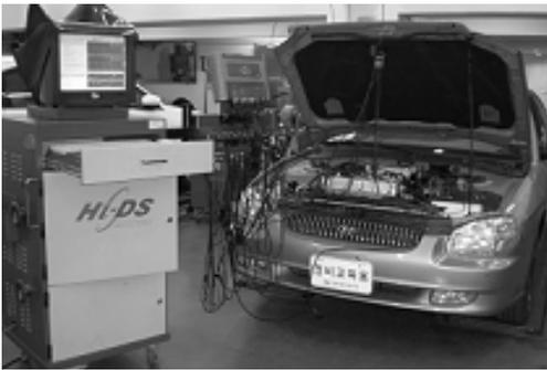
Photo 1. Engine tune-up tester for engine sensors.
