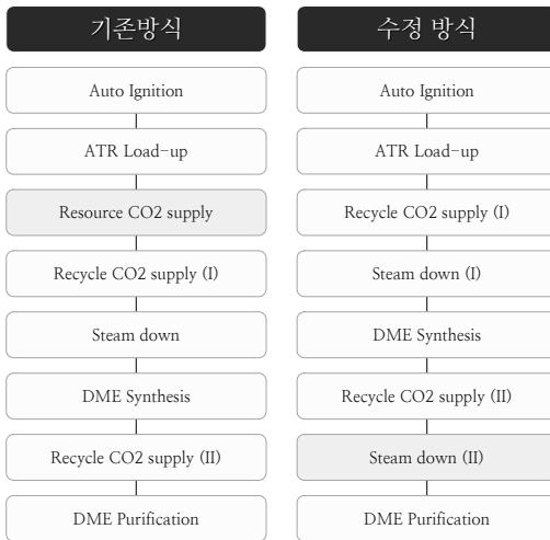
Fig. 3. Block diagram of operation method in DME synthesis process.
