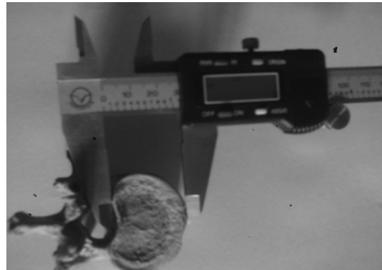
Fig. 5. Dimensions measurement with vernier caliper.
