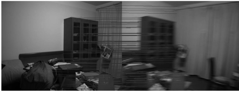
(b) The obtained feature matches in the bottom layer before applying RANSAC. There are 157 matches.
