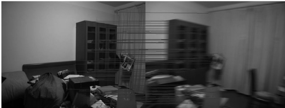
(c) The obtained feature matches in the bottom layer before after RANSAC. There are 95 matches.
