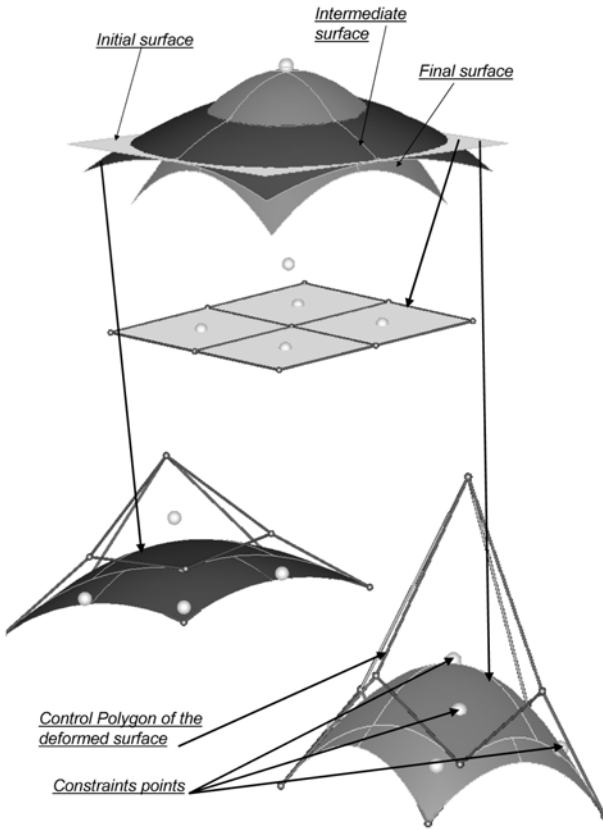
Fig. 5. Deformation of surface by energetic method
