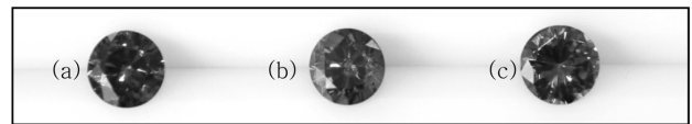
Fig. 3. Photographs of round brilliant cut of cobalt (II) cobalt (III) oxide (0.5 mol%, identical) and cerium (IV) oxide ((a) 0.3, (b) 0.33 and (c) none) doped YSZ single crystals heat treated in nitrogen at 1200°C for 3 hrs.
