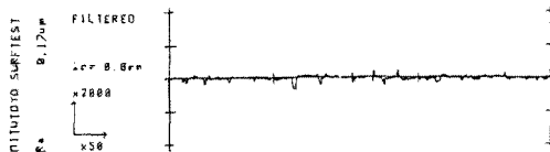
Fig. 15 Surface roughness after magnetic polishing (B=6,000G, V=1.46m/s, F=1.5mm/s, CBN)
