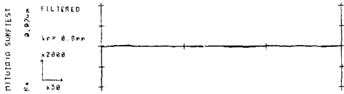
Fig. 14 Surface roughness after magnetic polishing (B=6,000G, V=0.73m/s, F=1.5mm/s, CBN)
