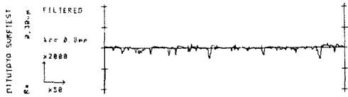
Fig. 13 Surface roughness after magnetic polishing (B=3,000G, V=0.73m/s, F=1.5mm/s)
