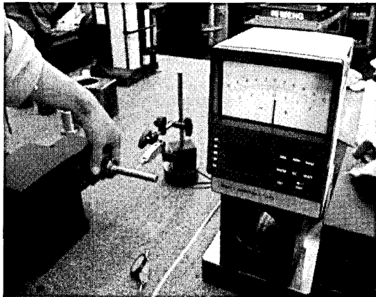
Fig. 13 Measurement of twisting deformation
