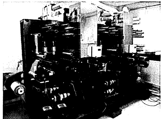
Fig. 3 Developed roll-to-roll printing system with multiple printing methods
