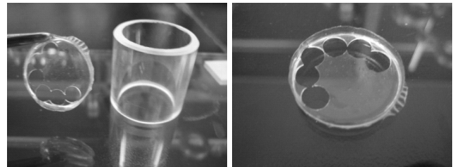
Fig. 1 A membrane prepared with a glass ring (left) and cut in a diameter of 4.0 mm (right).
