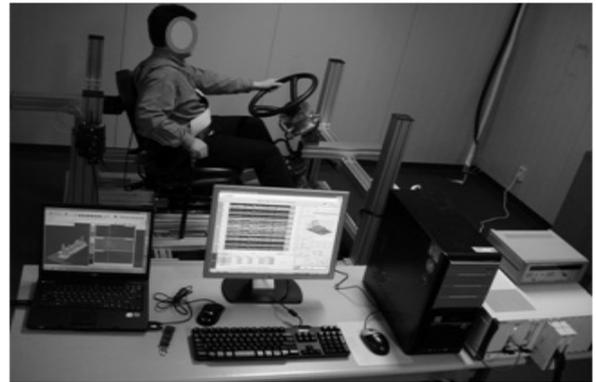
Fig. 5 Photo of measuring the seatbelt body pressure distribution on tractor seat simulator.
