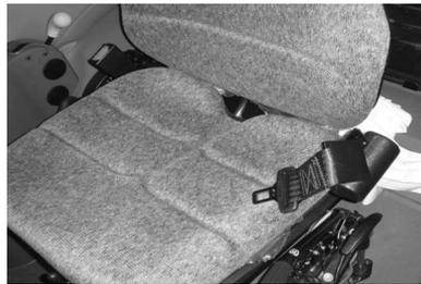
**Fig. 8** Retractable seatbelt.
