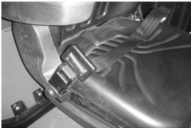
**Fig. 7** Non-retractable seatbelt.
