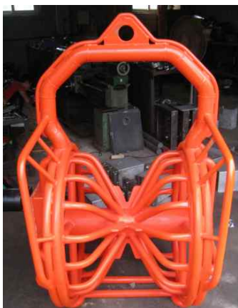
Fig. 10 Net hauler for fishing net washing
