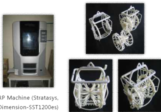
Fig. 9 Net hauler prototypes made by RP machine for verification of the structural design
