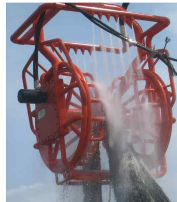
Fig. 12 Evaluation of new net hauler's performance for fishing net washing
