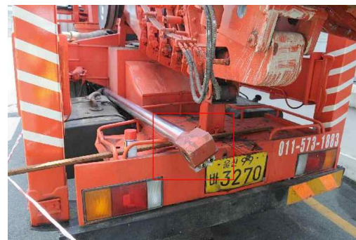
(c) Failure pin in the aerial lift
