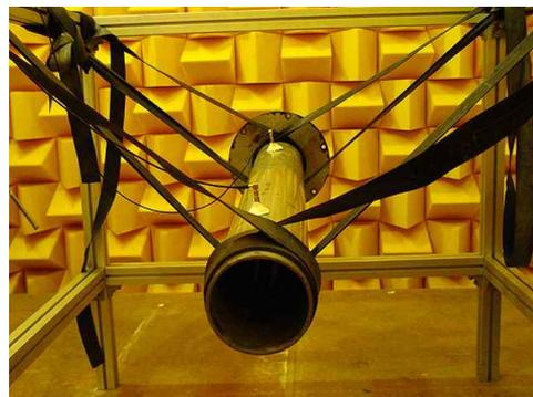
Fig. 5 Picture of the installed pipe in an anechoic room
