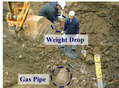
**Fig. 9** A buried real gas pipe test
