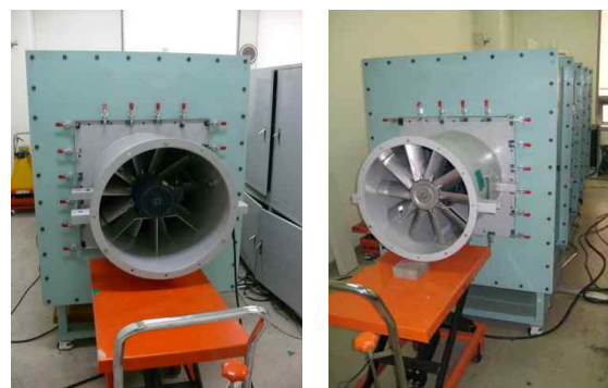
Fig. 6 Performance test of the ventilation axial-flow fan
