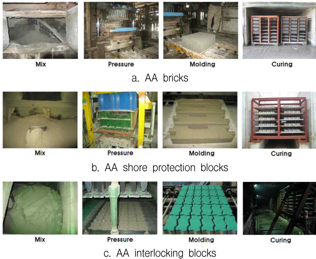
Figure 2. Production process of secondary products of AA concrete
