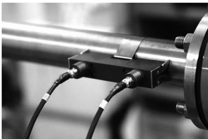
Fig. 4. Ultrasonic Water Meter attached on Pipes
