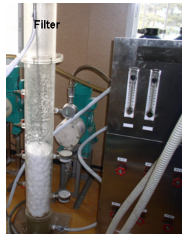
Fig. 1 Experimental setup of lab-scale filtration device
