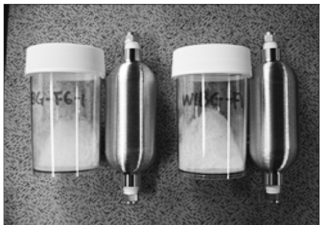
Fig. 2. Stainless steel bottle and glass powder sample for PCT test
