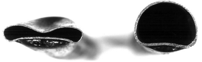
Fig. 6 Collapsed cross-sections of damaged tubes subjected to combined axial compression and external pressure
