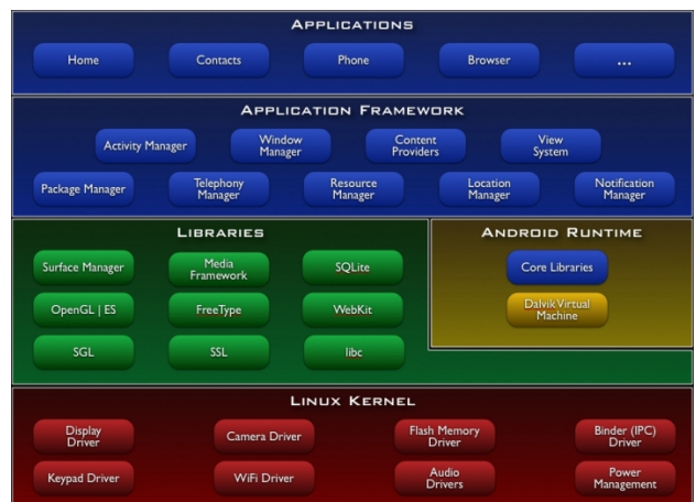
Fig. 6. Android Kernel, Important Components and API[13].
