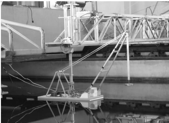
Fig. 7. 1/100 Scale floating crane model
