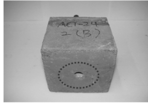
(c) Pullout failure
