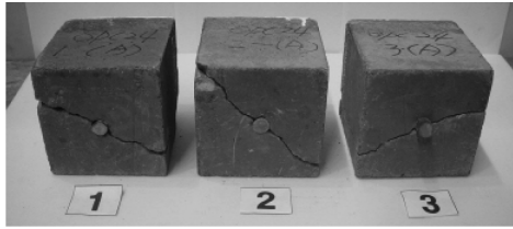
(a) Splitting failure
