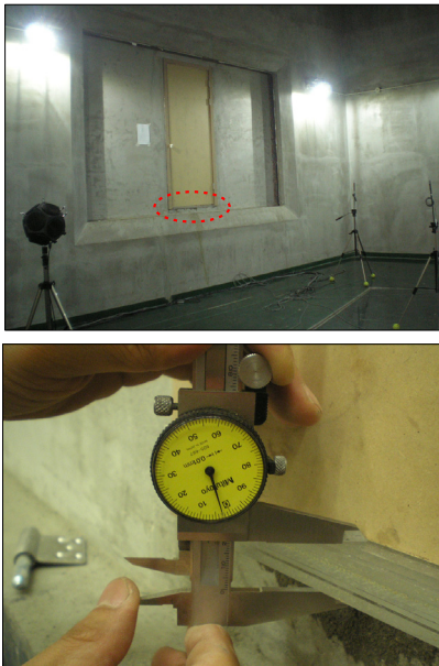
Fig. 2 Reverberation chamber and measurement of the thickness of acrylic plates to set the aperture
