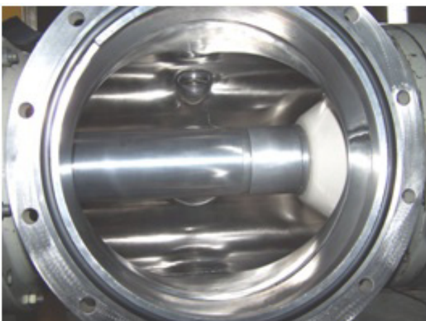
Fig. 1. Gas-insulated bus duct model under study.
