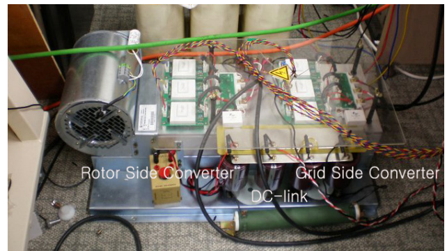
(b) An actual picture of the experimental setup
