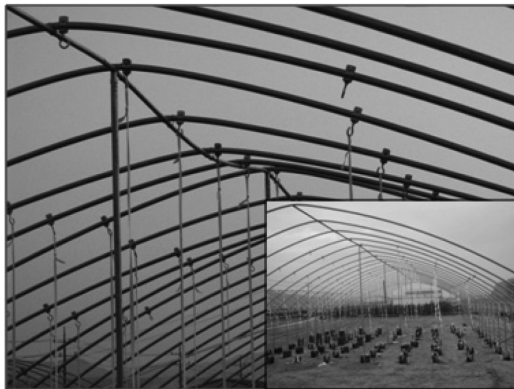
Fig. 7. A view of the static load test (Large photograph: under the maximum snow load of 24.1 cm, Small one: when unloaded after the last load) and displacement according to the snow load step for the 8.2 m single-span plastic greenhouse (SPVHS).
