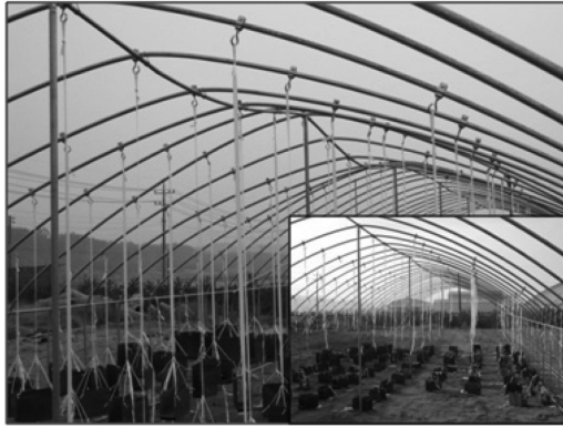
Fig. 6. A view of the static load test (Large photograph: under the maximum snow load of 35.5 cm, Small one: when unloaded after the last load) and displacement according to the snow load step for the 6m single-span plastic greenhouse (SPVHS).
