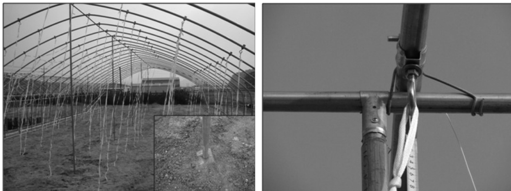
Fig. 3. The single-span plastic greenhouse with the pole and its bottom plate for load test.
