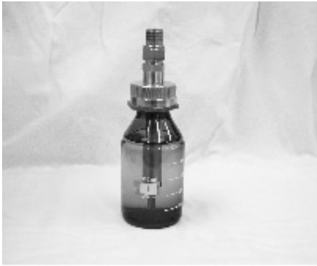
Fig. 2 Modular electrode probe bottle assembly.
