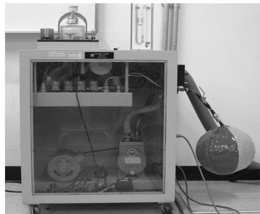
Fig. 1. The IEC type spark ignition test apparatus.
