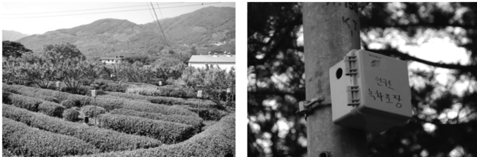
Fig. 2. Photographs of an automatic weather monitoring system (left) and instruments of air temperature and humidity (right).
