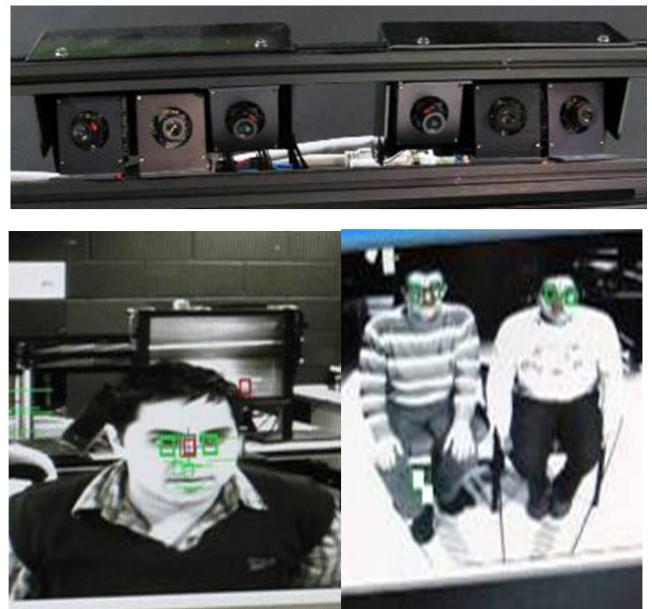
Fig. 9. Head tracker and output. The top figure shows the head tracker camera array. Six cameras are employed to track users from a 1,000-3,000 mm distance. The left picture shows the detection of a single user's eyes (smaller green rectangles), and the right picture, two users.
