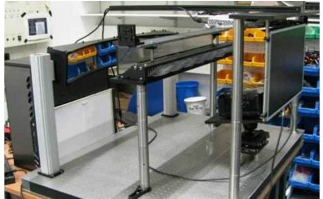
Fig. 1. Principal components of the MUTED prototype: 120Hz DLP projector, 120Hz LCD, field mirror, vertical diffuser, and a single array.
