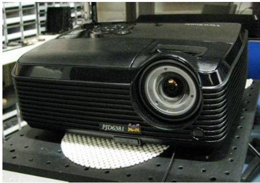
Fig. 4. ViewSonic 120Hz Conventional Projector. Provides a backlight for a direct-view LCD by producing a spot pattern controlled by the head tracker and MUTED optics.
