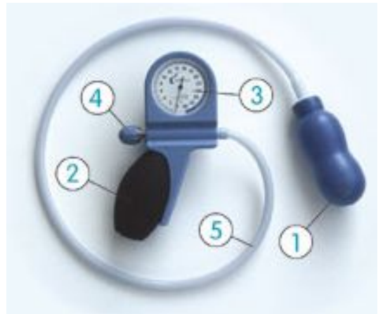
Fig 1. Perineometer. consists of (1) a narrow contoured silicone balloon and introducer, (2) a hand pump, (3) a pressure display, (4) an air release valve, (5) connected by a flexible plastic tube
