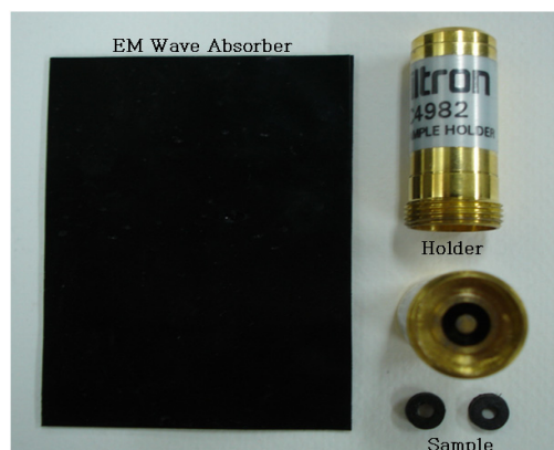
Fig. 4 A photo of EM wave absorber, Sample Holder and Sample
